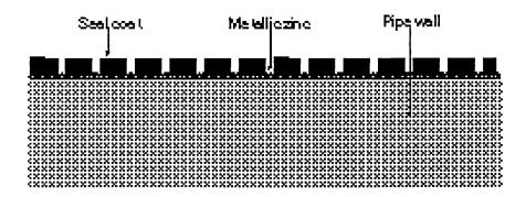
The zinc is factory applied to a clean and dry pipe surface, usually just after the ferritisation heat treatment of the pipe. The zinc coating is generally applied by the technique of electric arc guns, in other words the molten metal is sprayed on the pipe after an electric arc is drawn between two zinc wires. Other techniques can be used to obtain an equivalent coating: flame spray, spray of molten zinc from a bath.
