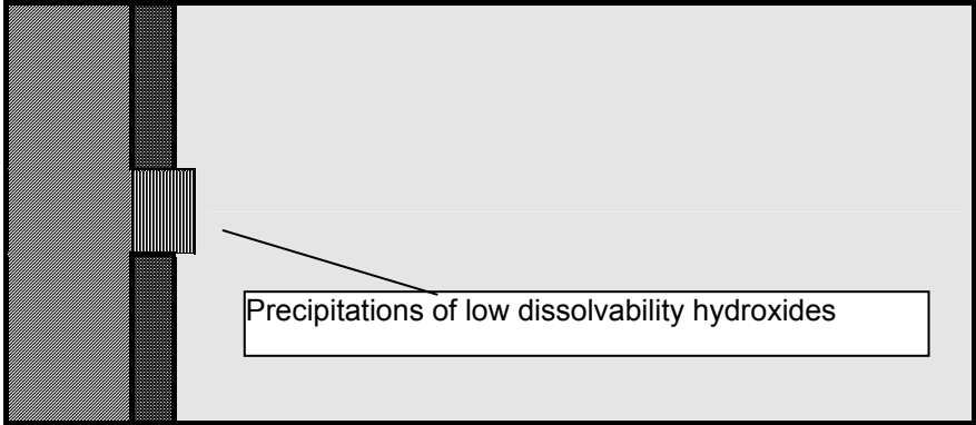
Fig. 2.4 Soil water with only salts of earth alkaline metals. Precipitation of low-dissolvability hydroxides of earth alkaline cations at the metal / electrolyte phase boundary
