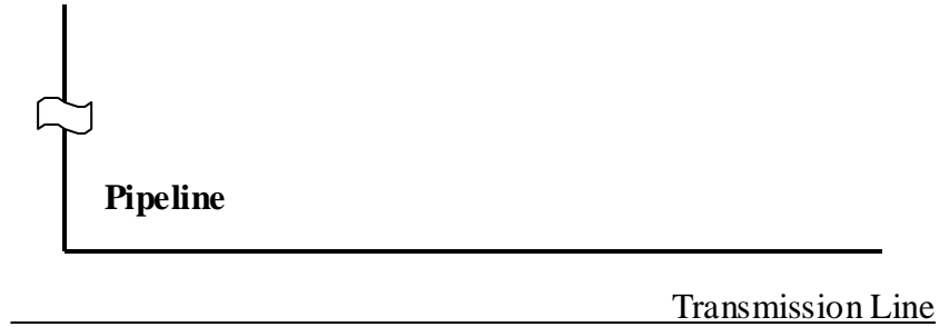
FIGURE 7 – Case 2 : The pipeline extends beyond the parallel routing at one extremity and stops at the other extremity without earthing.
