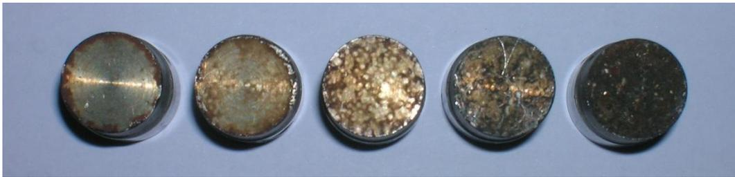
Fig. 3: Coupons of type 2 (after removing the surrounding polymer) after 3 months test in the series of 14 V avg a.c. voltage in soil solution with 17  $\Omega\text{m}$ . The coupons correspond from left to right to the series 1 to 5.
