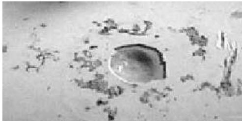
**Figure 3 - Typical a.c. corrosion on an FBE coated pipeline (Reference 7)**
