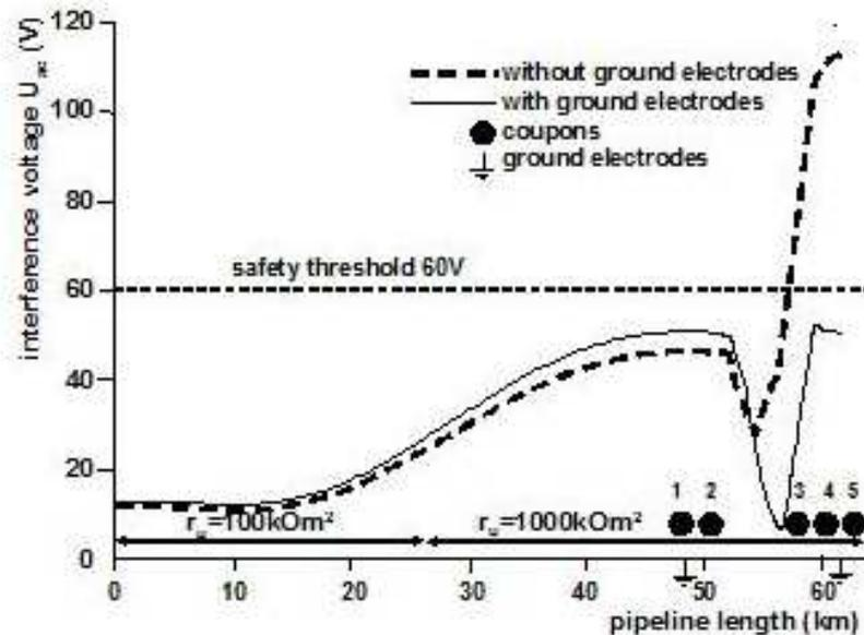
Figure 4:  $U_{a.c.}$  along a pipeline, DN 500, built in 1999
