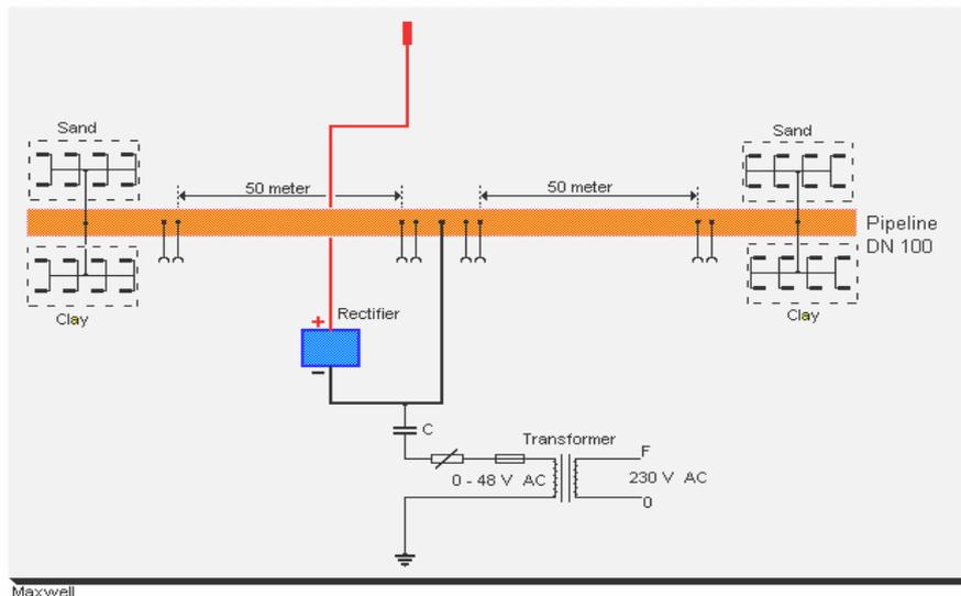
**Figure 1.** The field test plant with its electrical installations and buried test coupons.
