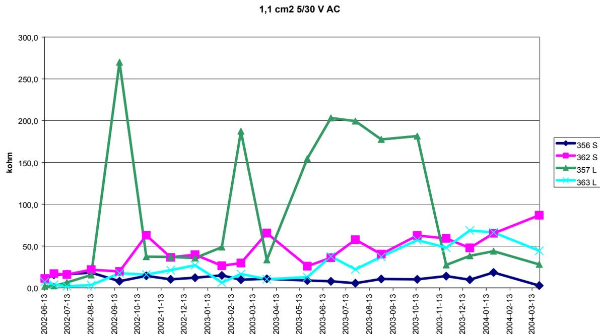
**Figure 3:** The resistance between steel surface and earth for four coupons (1,1 cm<sup>2</sup>) in sand (S) and clay (L).
