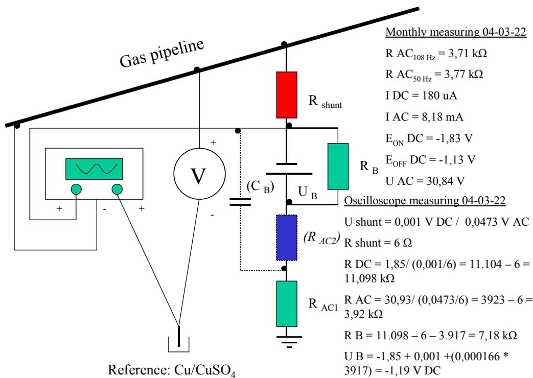
**Figure 5:** The Battery model
