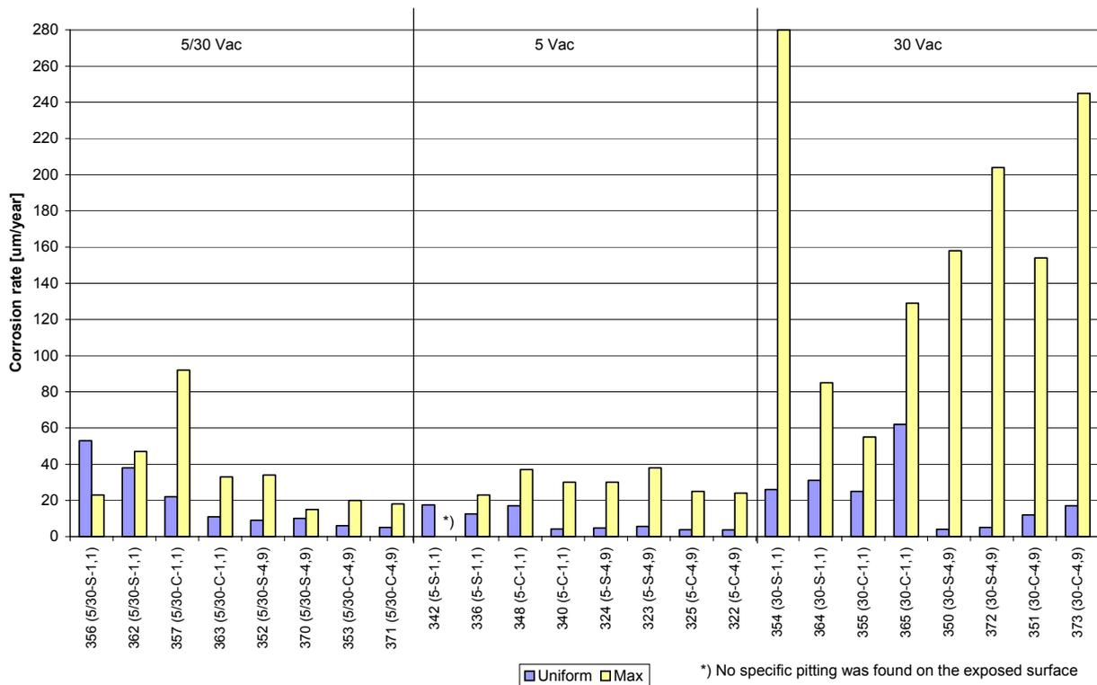
**Figure 2:** Uniform and maximum local corrosion rates on the test coupons in the 5/30 V<sub>AC</sub>, 5 V<sub>AC</sub> and 30 V<sub>AC</sub> test series.
