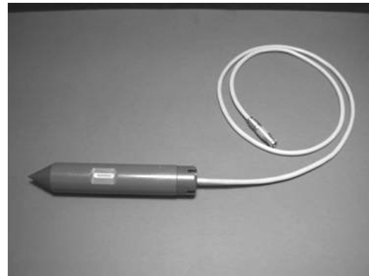
Figure 5. ER coupon for corrosion rate measurements.
