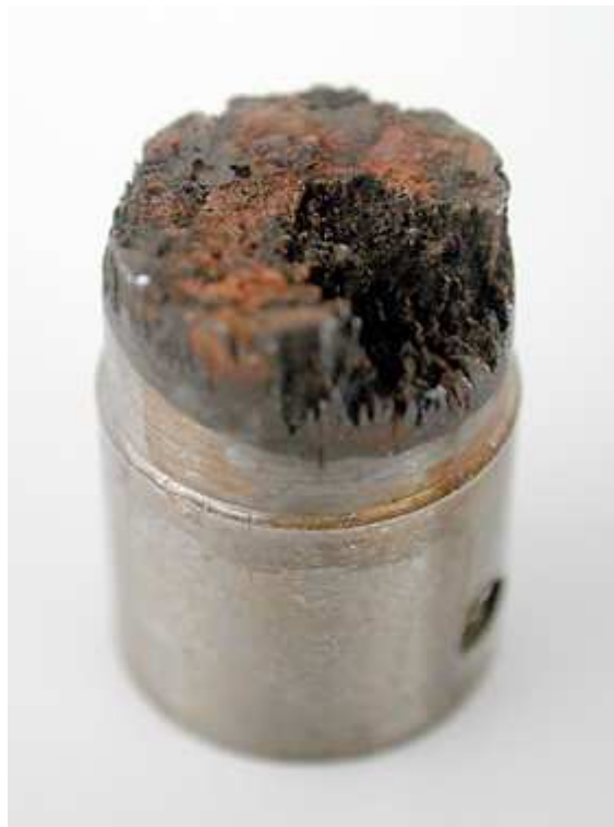
Fig. 7: Corrosion attack on a field sample The diameter is 11.5 mm.
