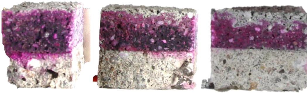
Figure 2: a) Realkalization after 35 days storage under 100 % RH , b) subsequent dry storage under 60 % RH after 28 days , c) subsequent dry storage at 60 % RH after 112 days
