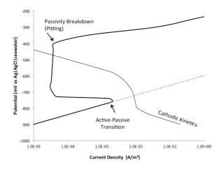
Figure 9 Schematic E-Log |i| Diagram for Passivity
