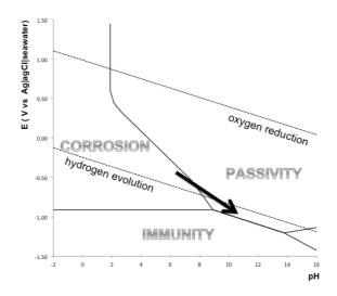
Figure 8 Schematic Poubaix Diagram for Passivity under CP.
