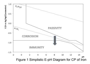
The arrow in this figure suggests that the potential is shifted from the zone where corrosion is the thermodynamically favoured outcome to the zone of immunity, where iron is stable. At first sight this interpretation of CP aligns with Pourbaix's view that CP... is based on the fact that the potential of iron is lowered, on reduction, into the domain of immunity in which the corrosion of iron is theoretically impossible [3].
