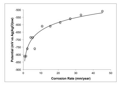
Figure 4 Corrosion Rate vs Potential: Steel in 0.1M HNO<sub>3</sub> [27]
