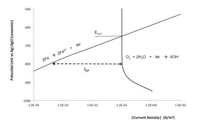
Figure 2 Electrode Kinetic Theory for CP (Activation Control)
