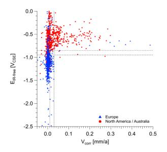
Figure 7 Site Data: Potential versus Corrosion Rate (Reproduced from [42])
