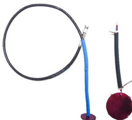
Figure 4: Ag/AgCl and Cu/CuSO 4 Reference (Electrode) Probes
