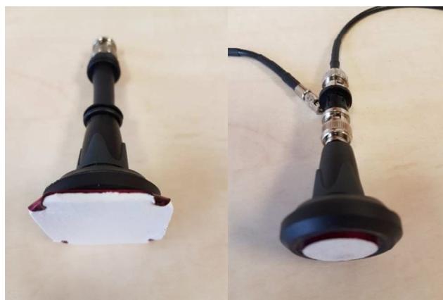
Figure 6: Ag/AgCl and Cu/CuSO 4 Reference (Electrode) Probes
