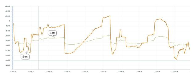
While in the first case a passive film has been formed on the metallic surface (Eoff is about -1,2 VCSE), thus protecting from corrosion during short duration anodic interferences, in the second case no enough current is reaching the metallic surface of the coupon (Eoff is about -0,85 VCSE) thus meaning an immediate corrosion process activation as just as current moves anodic.
