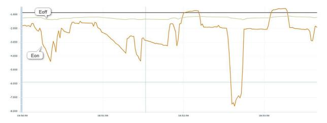
The second graph shows the evolution of an Off potential that changes significantly with respect to On potential variations: in this case, it can be assumed that no
