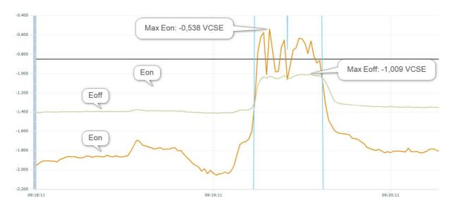
The Eoff measure on coupon shows in both cases the presence of an already strong overprotection condition, so demonstrating that not only it is not necessary to increase cathodic protection current, but that should be even evaluate the possibility of reducing it.
