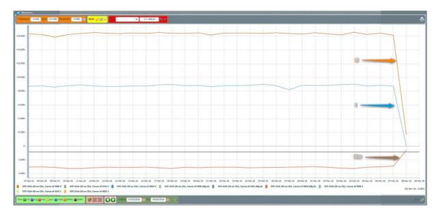
Remote monitoring device are usually connected to the same main power of the rectifier: this allows to detect immediately the main power failure, sending an alarm to the operators. Below is the trend over time of the battery level of the remote monitoring device, which is powered by a power supply and equipped with backup batteries in the absence of an external power supply.
