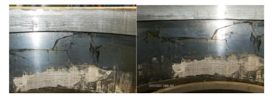
In the following picture we can witness the mechanical damage that was caused by the repetitive lightning strikes.
