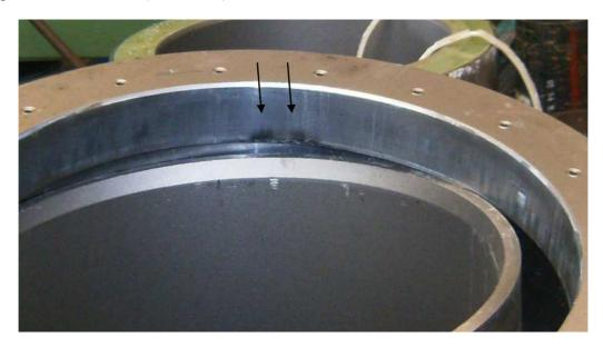
An other view of the IJs main body proves the existence of lightning sparkovers. The shape of the burnings proves indeed that the cause was surge/lightning currents.
