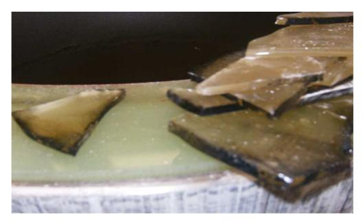
It is obvious that all insulating properties are lost and that the IJ has been susceptible to non-desirable effects; i.e. further mechanical damage with worst case senario the creation of arcs when lightning strikes occur.
