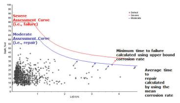
Intelligent PIG Inspection – Typical elaboration of the results
