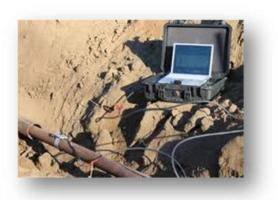
The method is able to reliably detect cracks and general metal loss along a short section of pipe. The method is very useful in Compressor Stations or Pumping Stations, where many pipes cannot be inspected with other techniques.
