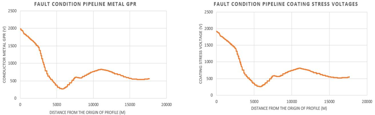
**Figure 5: Pipeline Metal GPR & Coating Stress Voltage- Phase to Earth Condition**
