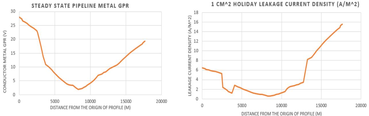
**Figure 4: Pipeline Metal GPR & AC Leakage Current Density - Steady State Condition**
