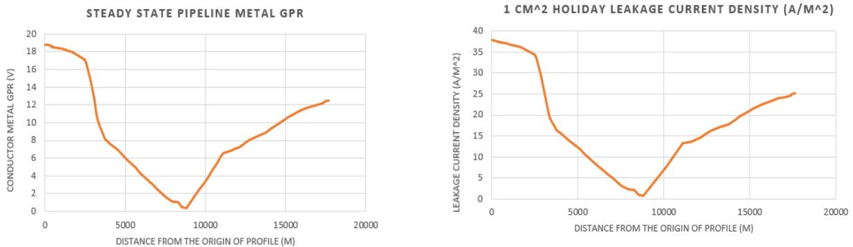
**Figure 2: Pipeline Metal GPR & AC Leakage Current Density - Steady State Condition**
