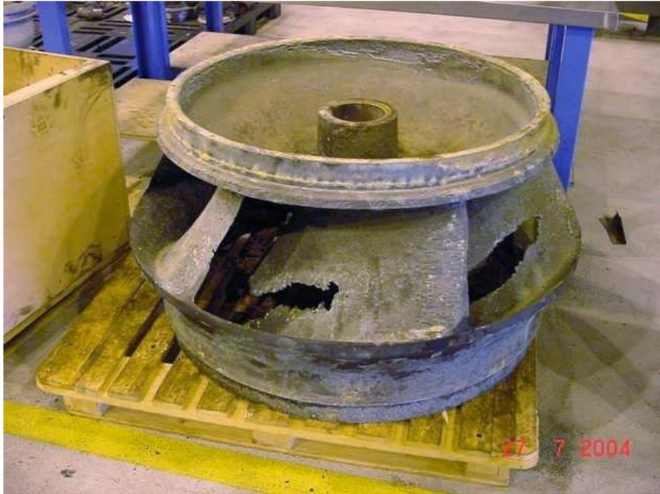
FIGURE 3 An NAB impeller suffering severe erosion corrosion due to sulphides.
