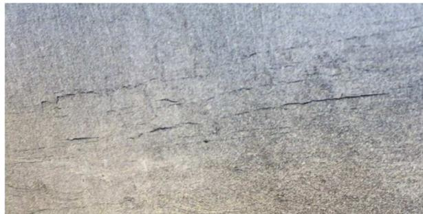
*Figure 5, Longitudinal linear indications, with the longest one being 140mm.*
