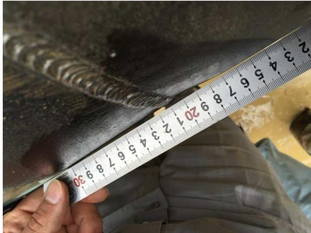
Figure 8, 4.25mm dent near weld between 9 – 11 o'clock position
