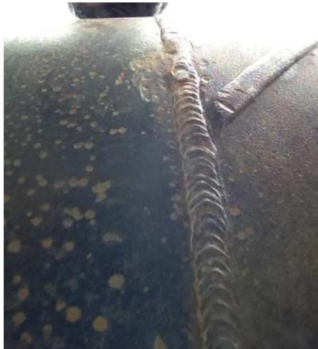
Figure 9, Pitting next to a girth weld because of presence of water under coating due to mismatch.
