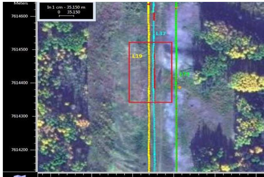
Figure 6, Blue pipeline route shows a lateral deflection from a straight line due to landslip.
