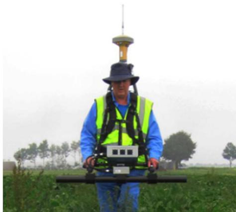
*Figure 1. scanner remotely collecting pipeline and positional data*
