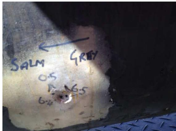
Figure 3, External corrosion metal loss with 26% wall thickness reduction
