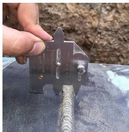
Figure 7. 2mm mismatch at a girth weld.
