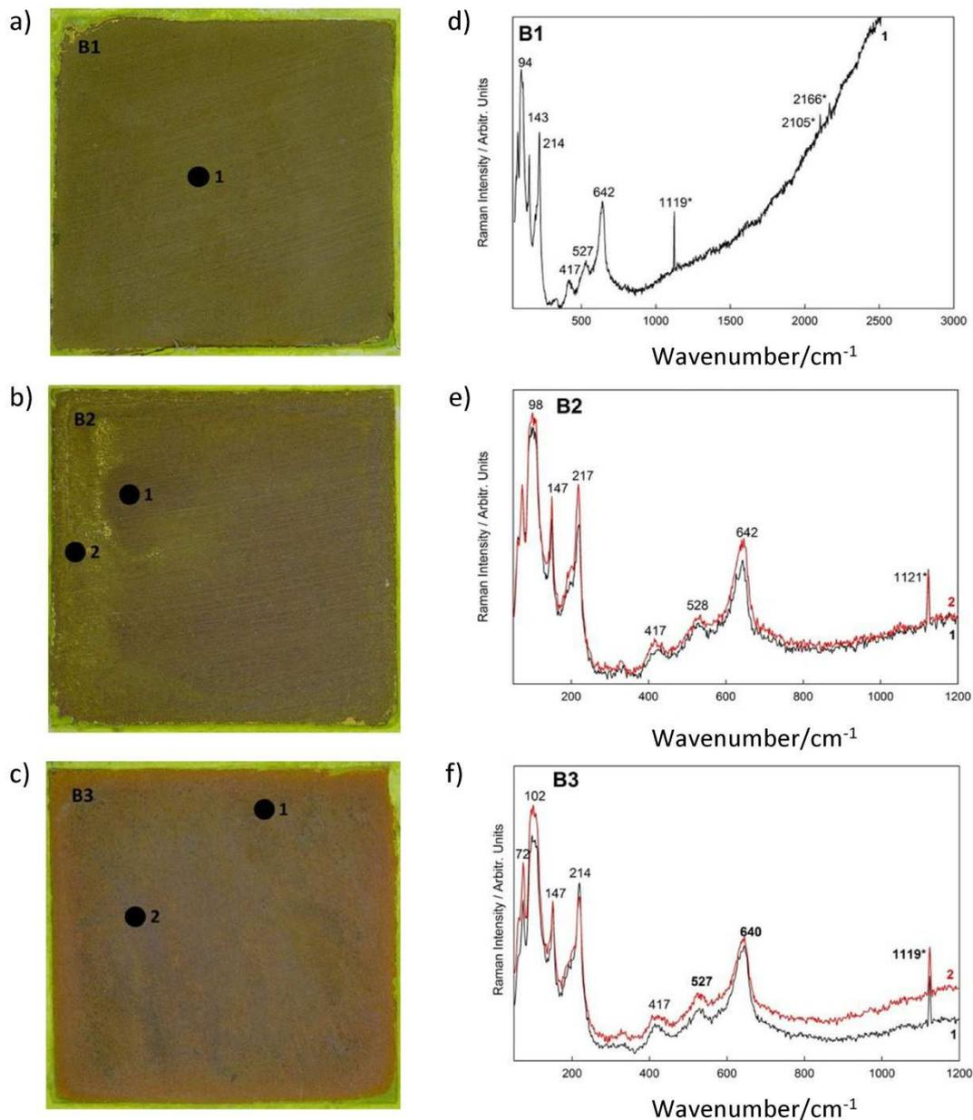
Figure 6: Images of non- approved brass (B1, B2, B3) after 44 weeks of exposure and Raman analysis
