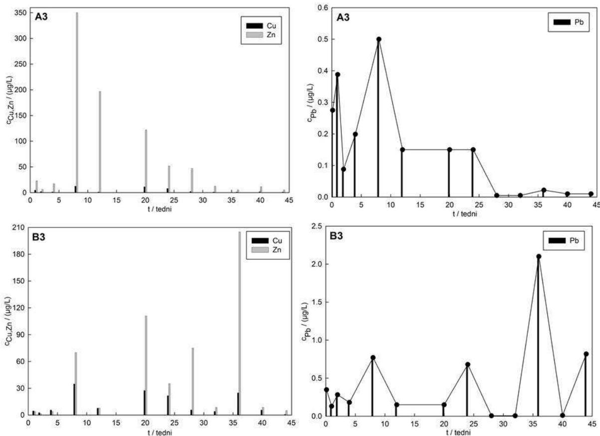
Figure 3: Concentration of zinc (Zn), copper (Cu) and lead (Pb) for 4MS approved brass (A3) and non-approved brass (B3) immersed in soft alkaline water pH 8.4
