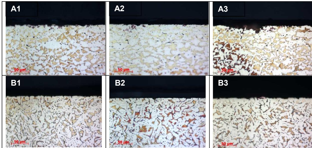
Figure 4: 4 MS approved brasses (A1, A2, A3) and not approved brass (B1, B2 and B3) after 44 weeks of exposure to different synthetic waters
