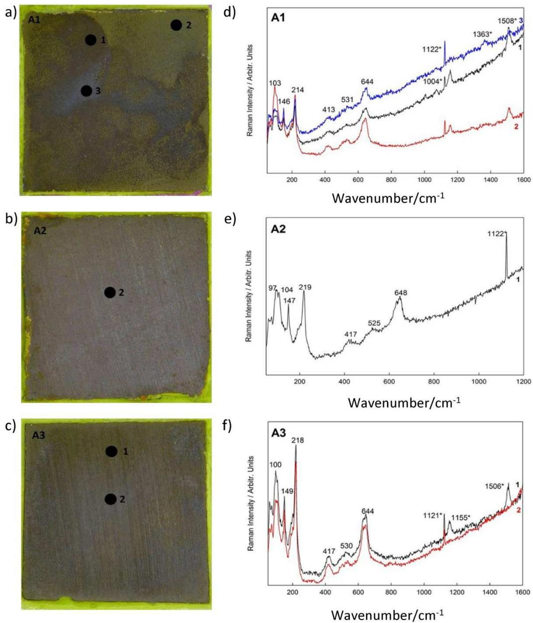
Figure 5: Images of 4 MS approved brass (A1, A2, A3) after 44 weeks of exposure and Raman analysis
