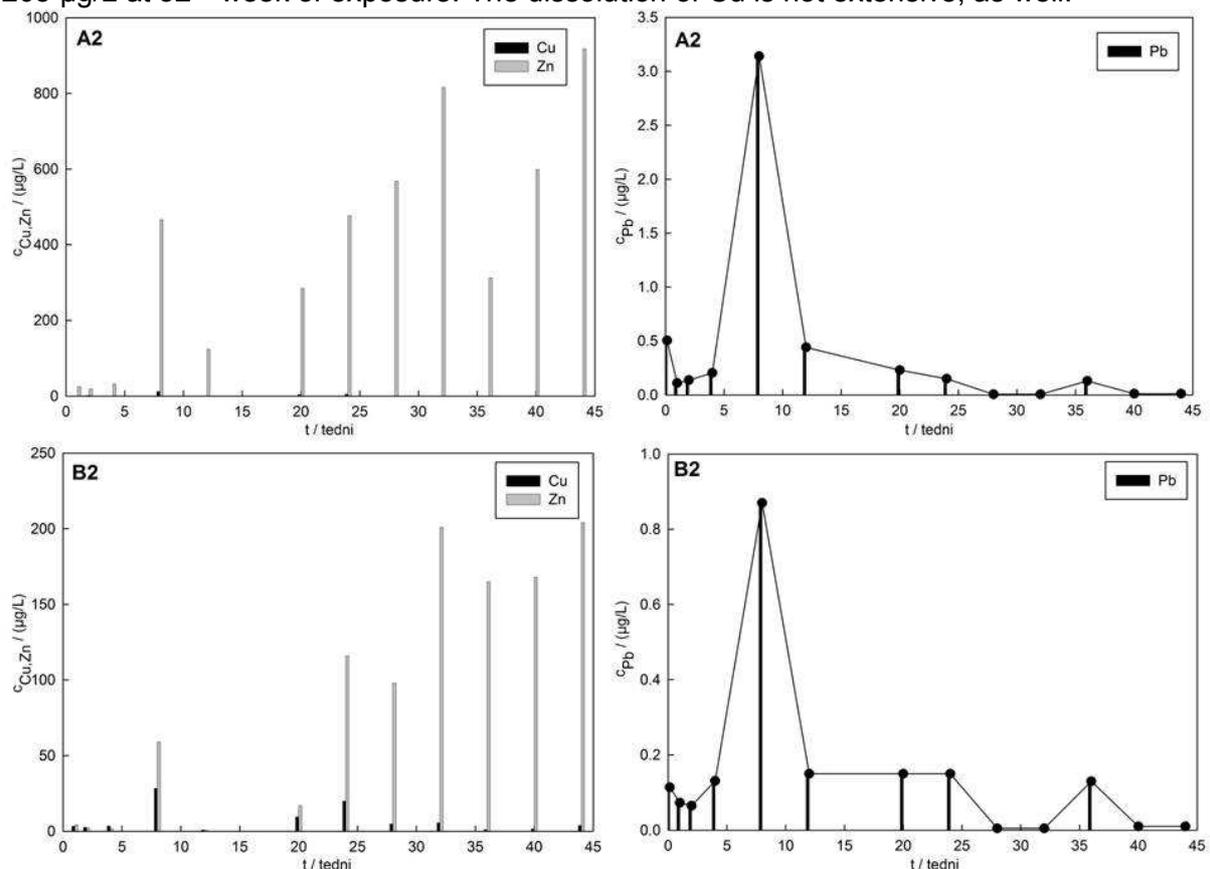
Figure 2: Concentration of zinc (Zn), copper (Cu) and lead (Pb) for 4MS approved brass (A2) and non-approved brass (B2) immersed soft acidic water pH 6.7
