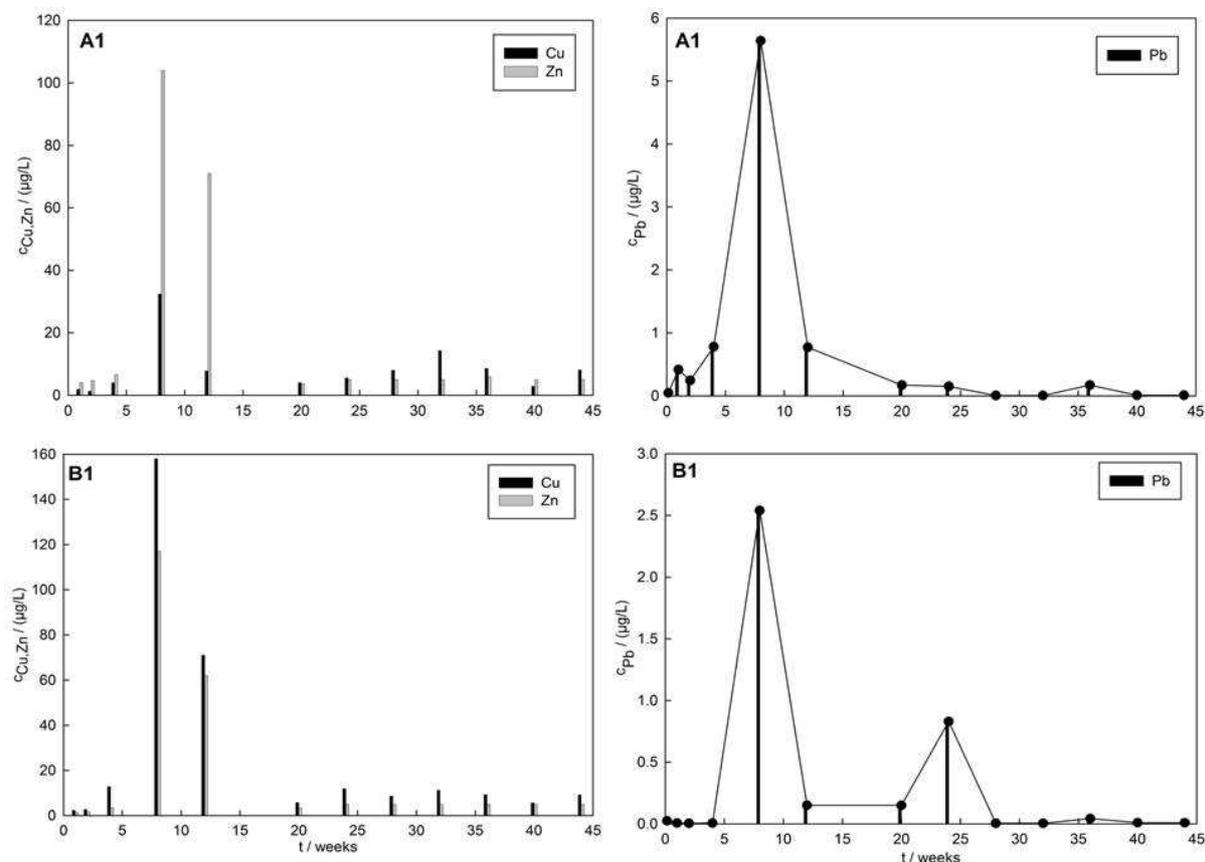
Figure 1: Concentration of Cu, Zn and Pb for 4MS approved brass (A) and non-approved brass (B), immersed in neutral alkaline water, pH 7.1
