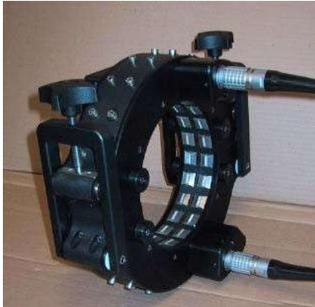
a – Guided Ultrasonics solid transducer system
