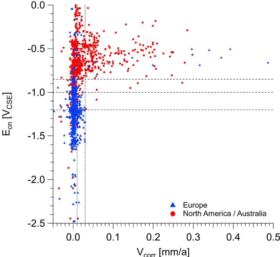
**Figure 3: Relation between on-potential ( $E_{on}$ ) and corrosion rate ( $v_{corr}$ ).**
