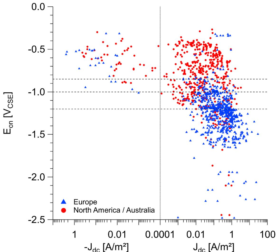
**Figure 1: Relation between on-potential ( $E_{on}$ ) and current density ( $J_{dc}$ ). Cathodic current has a positive sign.**
