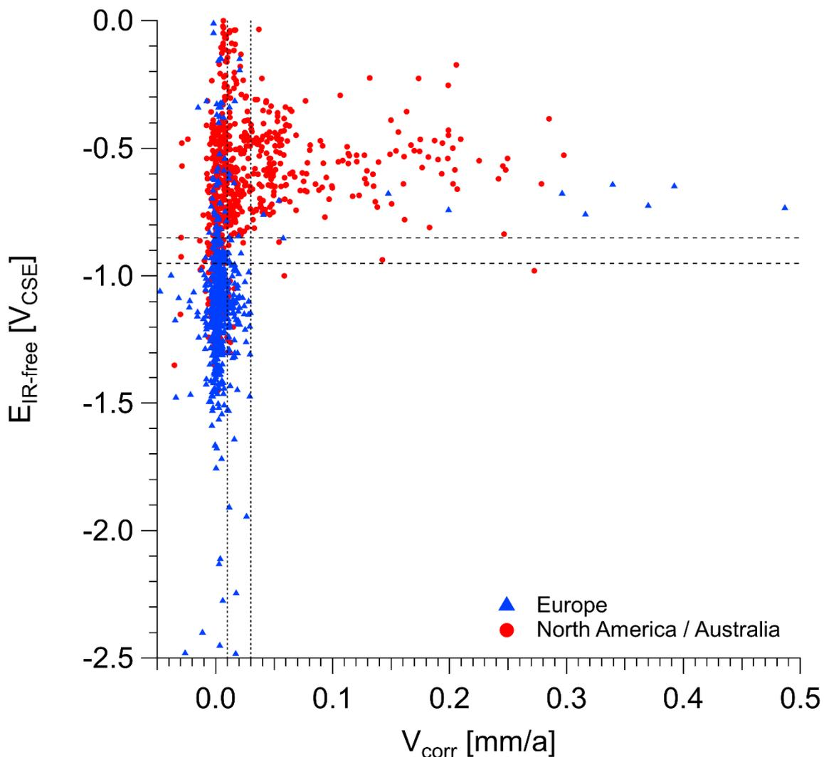
Figure 2: Relation between IR-free-potential ( $E_{IR-free}$ ) and corrosion rate ( $v_{corr}$ ).
