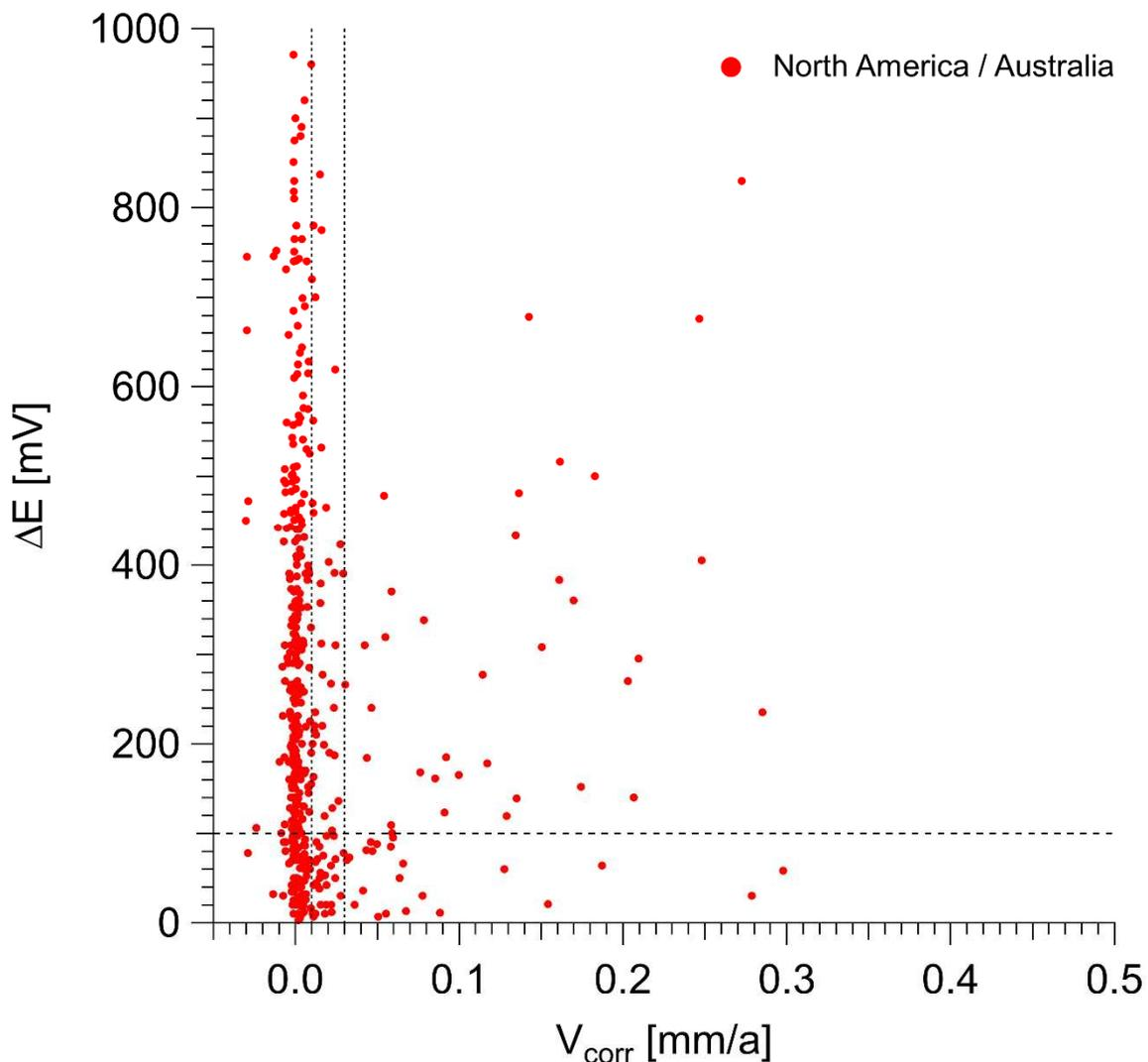
Figure 4: Relation between depolarisation ( $\Delta E$ ) and corrosion rate ( $v_{\text{corr}}$ ).
