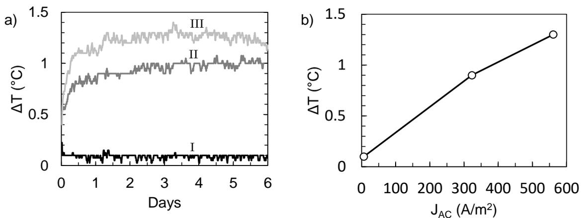
Figure 7: Temperature monitoring of the probe surface (5 mm) showing a negligible temperature change as a function of  $J_{\text{AC}}$ .
