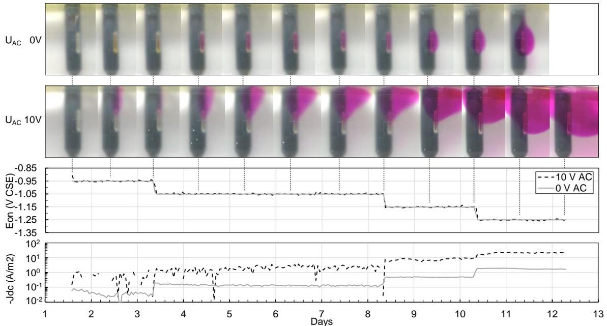
Figure 5: Visualisation of the an evolving pH > 9 environment in front of a steel surface at increasingly negative potentials from -950 mV to -1250 mV (CSE) with or without an AC perturbation. The higher DC current, caused by faradaic rectification of the AC current, is directly related to the cathode reaction and OH<sup>-</sup> development.
