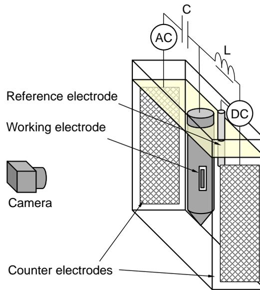
Figure 3: Experimental setup for visualisation of pH evolution at an electrode under AC and DC influence. The electrolyte is a transparent slurry simulating wetted sand, containing a phenolphthalein pH indicator with a transparent to pink colour change at pH > ~9.
