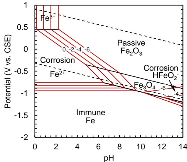
Figure 1: Calculated Pourbaix diagram for 25°C and 1 bar pressure. The corrosive regions are highly dependent on the concentration of Fe in solution indicated by the  $\log([Fe])$  values.
