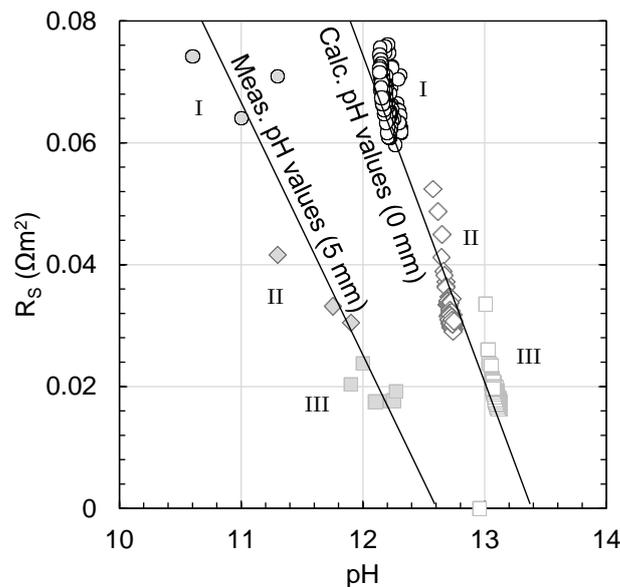
Figure 8: The effect of pH on the spread resistance caused by an increase of the ionic conductivity at the probe surface. Results from the measured pH values (trend line) as well as calculated pH values based on the DC current density and equation (4).
