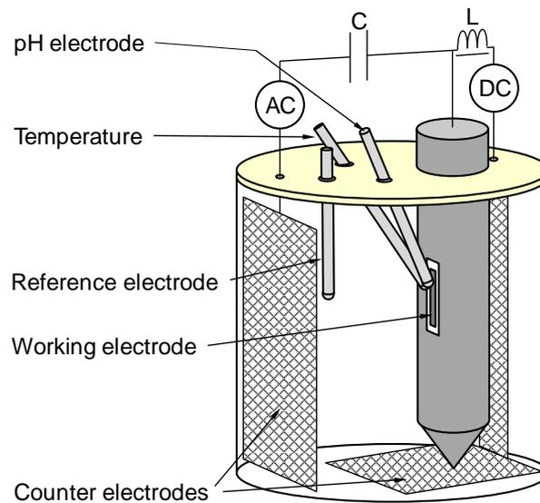
Figure 4: Experimental setup for monitoring of pH evolution at an electrode under AC and DC influence.
