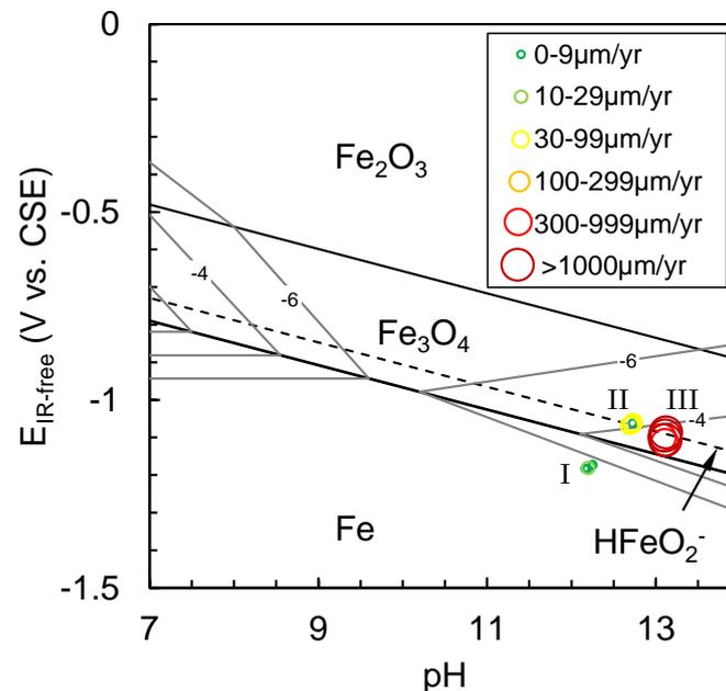
Figure 9: Corrosion rates plotted as points in the Pourbaix diagram at the corresponding calculated pH and measured  $E_{\text{IR-free}}$  value. High corrosion rates fall within the  $\text{HFeO}_2^-$  stability region. Without AC, the steel is in the immune region and no corrosion is measured.
