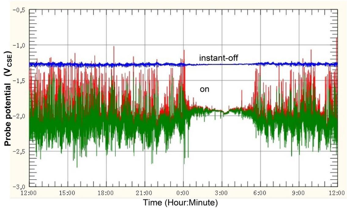
Figure 3 — Record of  $E_{on}$  and  $E_{off}$  during a period of 24h.
