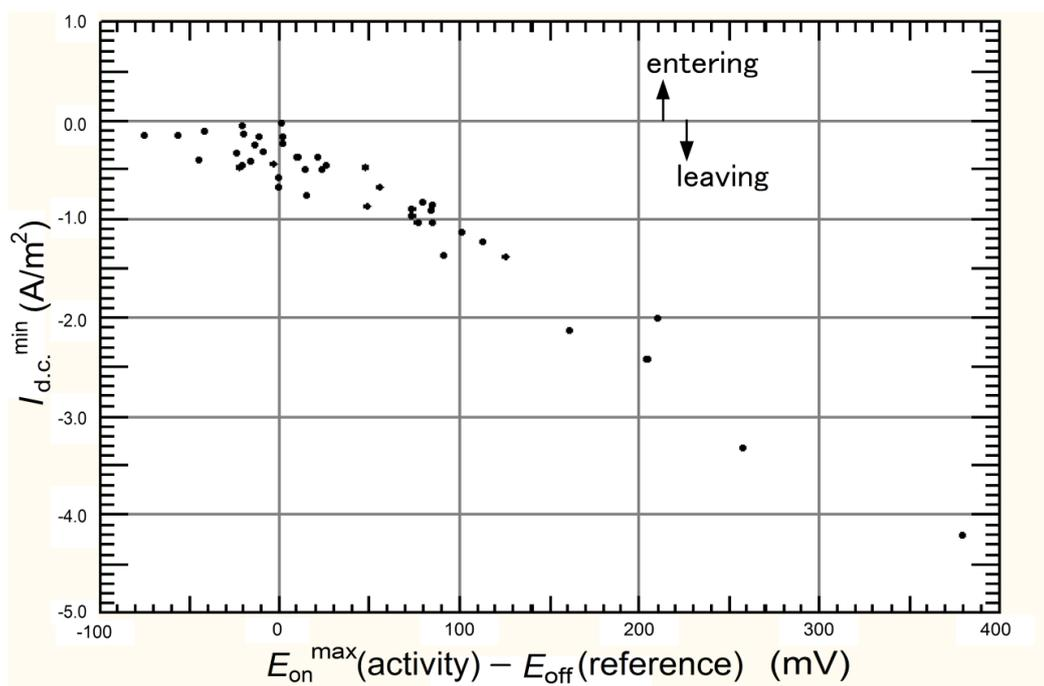
**Figure 5 — Relation between anodic shift ( $E_{\text{on}}^{\text{max}}(\text{activity}) - E_{\text{off}}(\text{reference})$ ) and  $I_{\text{d.c.}}^{\text{min}}$ .**
