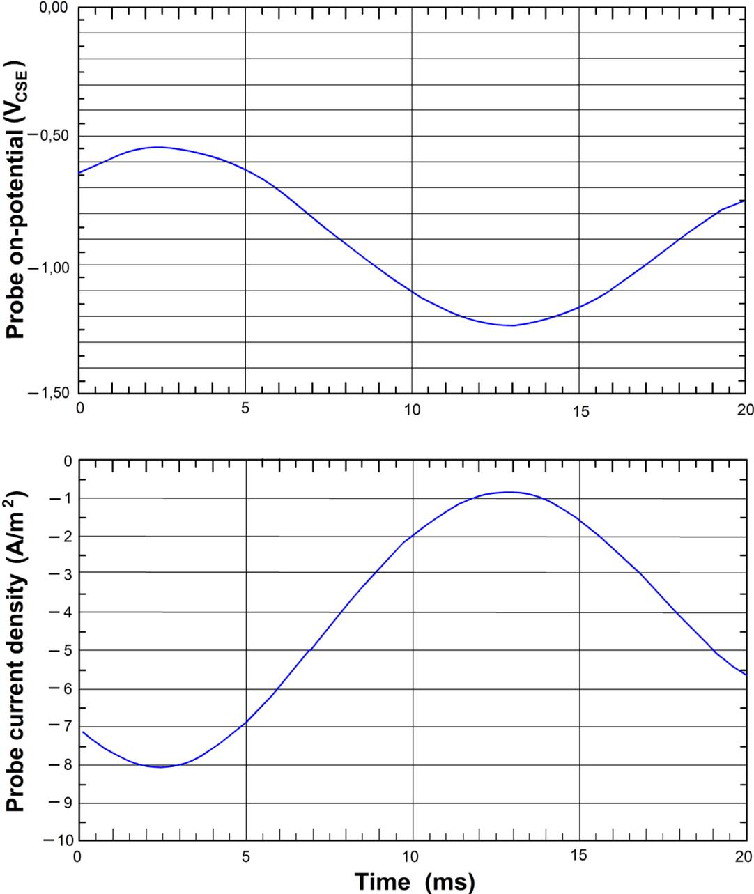
**Figure 6 — The most positive probe potential and the minimum probe current in 43200 units.**
