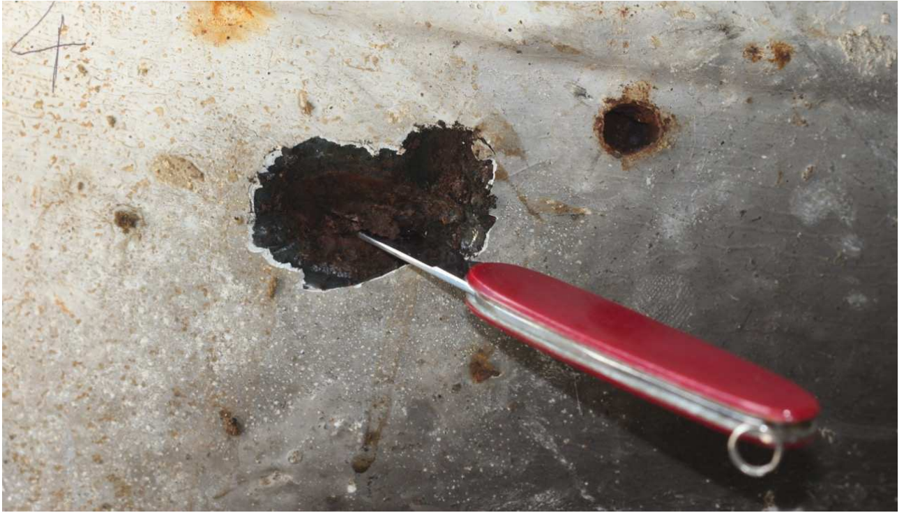
Corrosion pit beneath coating filled with corrosion product.
