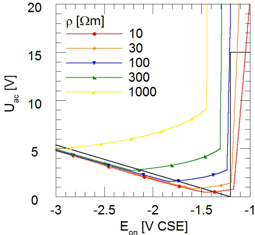
**Fig 2:** Influence of the soil resistivity on the limit value curve of a defect of  $1 \text{ cm}^2$  calculated taking into account the influences of thermodynamics, kinetics and mass transfer on the CP
