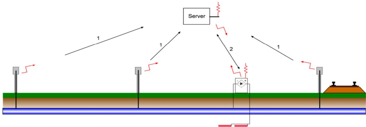
**Fig. 3: Structure of the control of the active CP**
