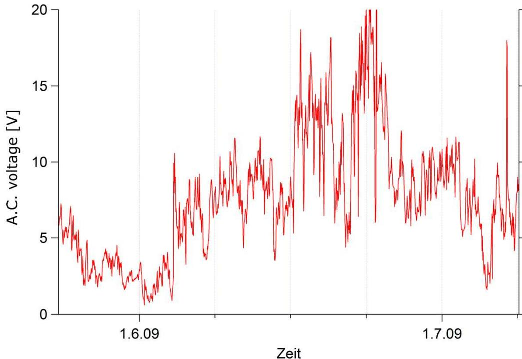
**Fig. 1:** a.c. voltage induced in the pipeline over a period of one month.
