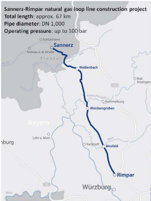
Figure 2: Line course LSR pipeline
