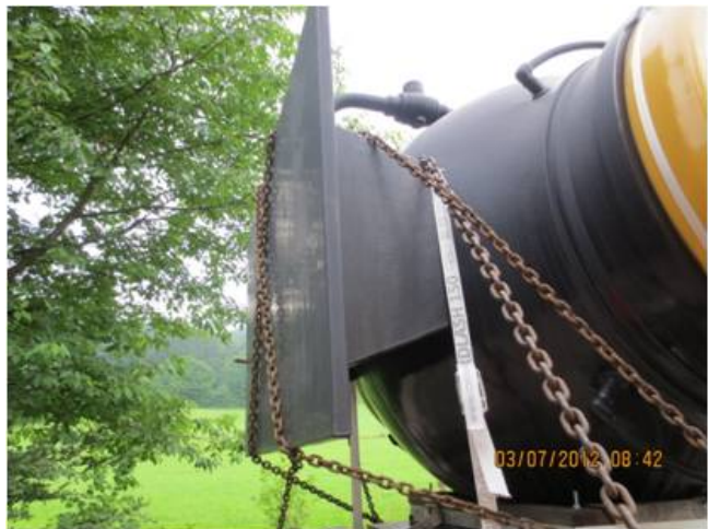
Figure 5: Coating damage during transport at valve support
