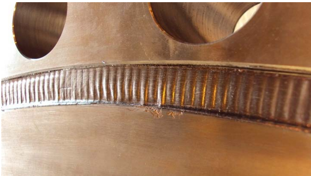
Fig. 1.5 : Female body with the graphite gasket ; Corrosion craters are visible near the gasket
