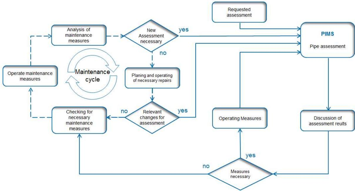
Figure 2: Involvement of the PIMS in a maintenance process
