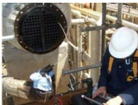
Figure 9 – .Application of guided waves on heat exchangers (a) and risers (b)
