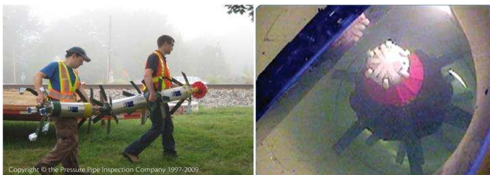
PipeDiver ® carried to insertion point PipeDiver ® at receiving point
