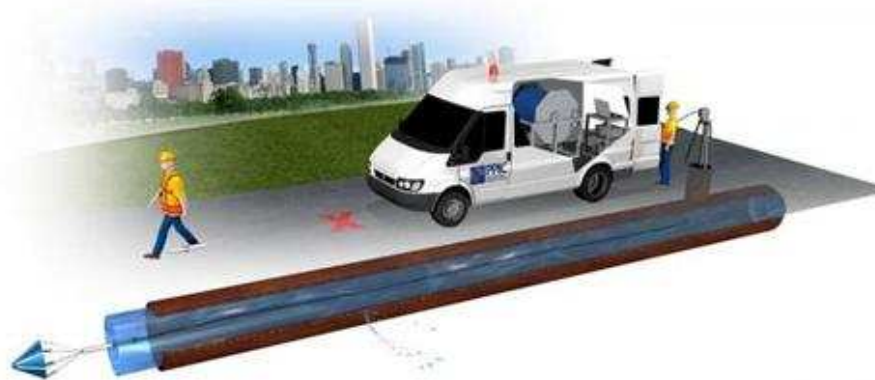
Principle of tethered inline leak detection Sahara ®
