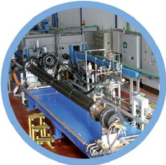
Fig. 4 Pipe expansion in Molecor® mould
