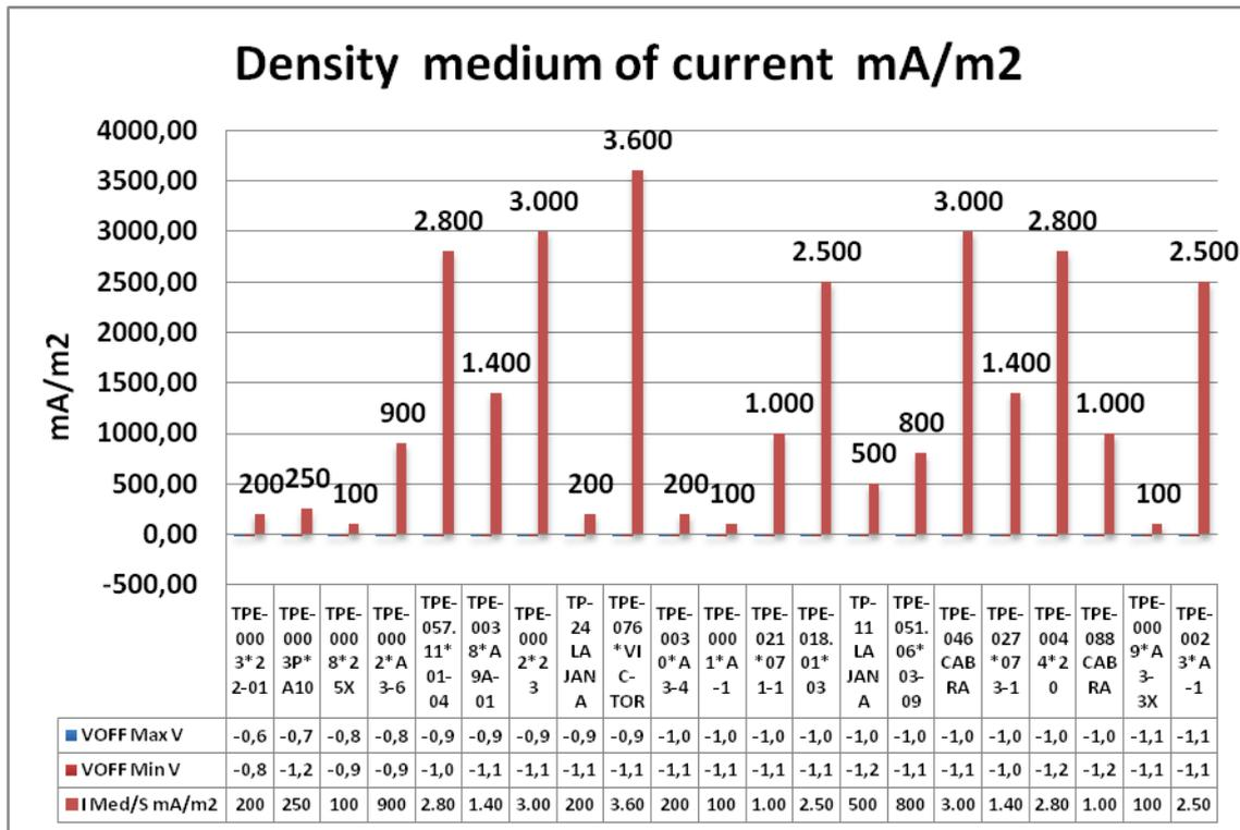
To know if there are a.c. interferences in the past 5 years we have been systematically performed instant measurements and data recordings of the a.c. voltage of the pipelines founding few cases with remarkable a.c. interferences. In those cases the adopted method was the installation of 1 cm<sup>2</sup> external potential test probes and draining systems to reduce the a.c. interference.
