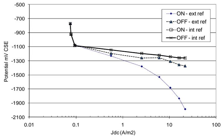
Figure 8. IR free potential tests using different potential probes.
