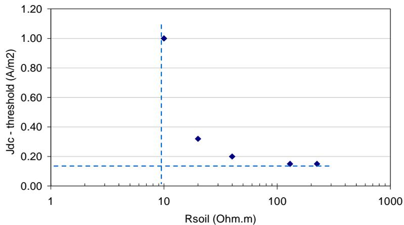
Figure 13. Threshold cathodic DC current density above which the spread resistance decreases – as a function of the soil resistivity [3].
