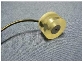
**1 cm<sup>2</sup> - test probe with internal luggin**
