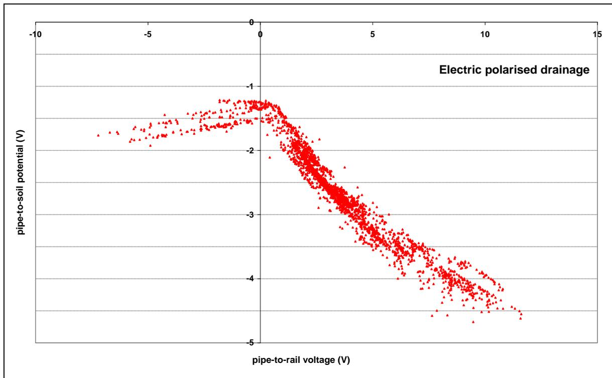
Figure 1 – Correlation between pipe-to-rail voltage vs. pipe-to-soil potential, measured via remote monitoring.
