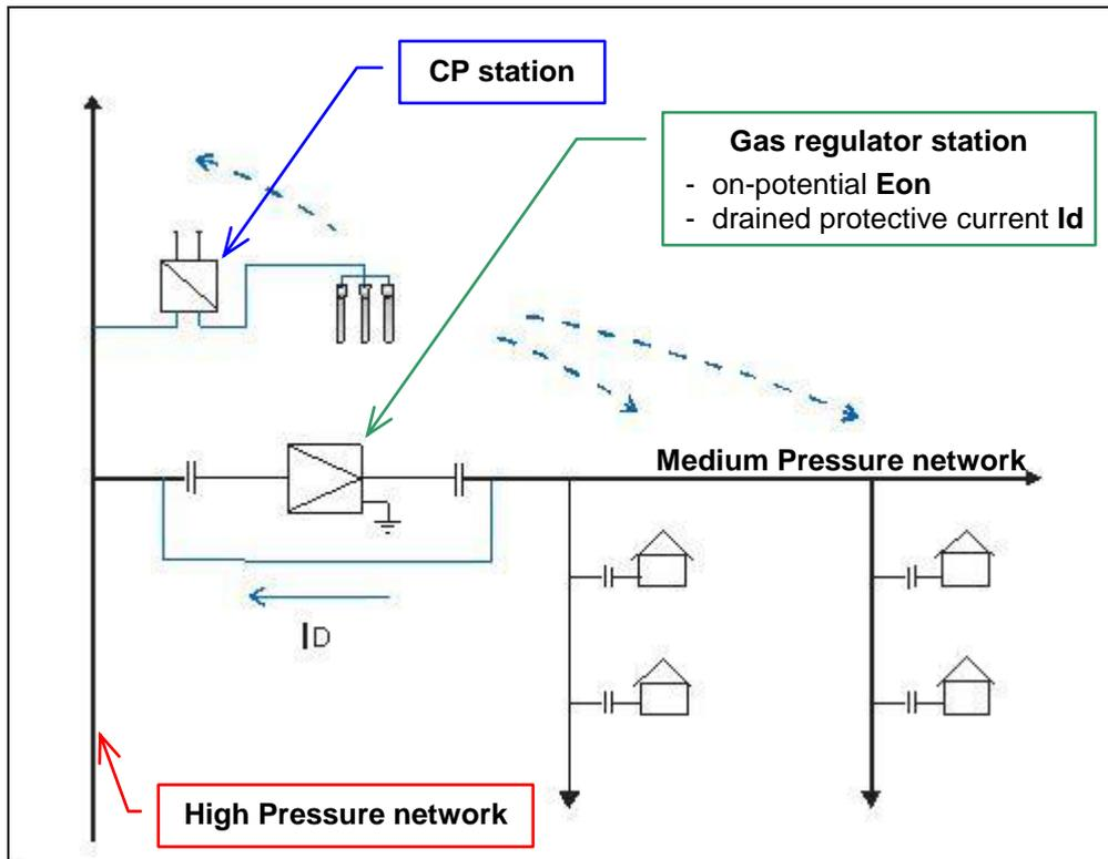
Figure 2 – Monitored interconnection point of two pipeline networks
