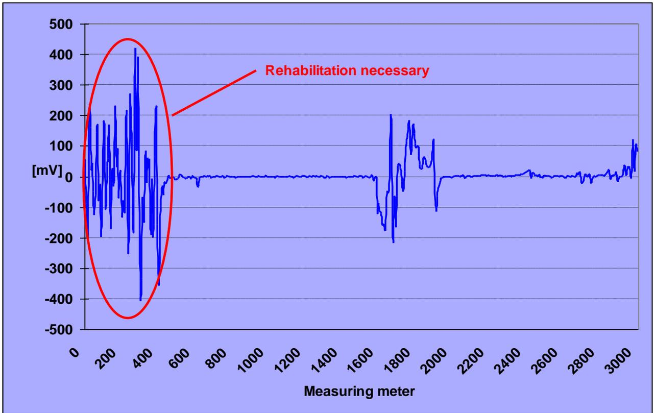
Figure 6: IFO measurement diagram prior to rehabilitation
