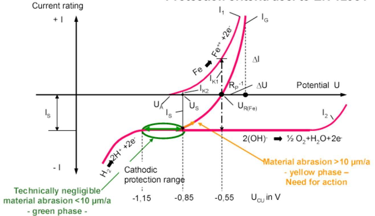
Figure 2: Current density potential curve of steel in vented and unvented soils
