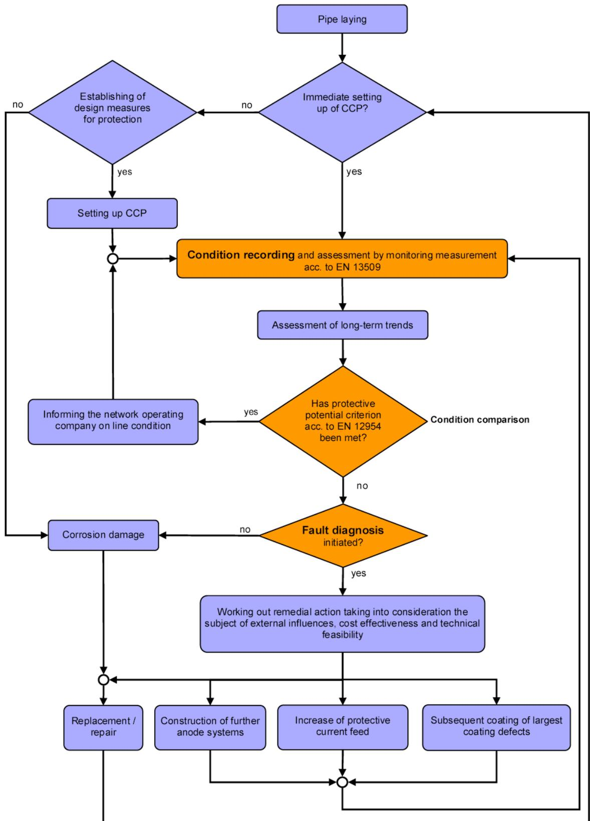
Figure 3: CCP-supported maintenance process
