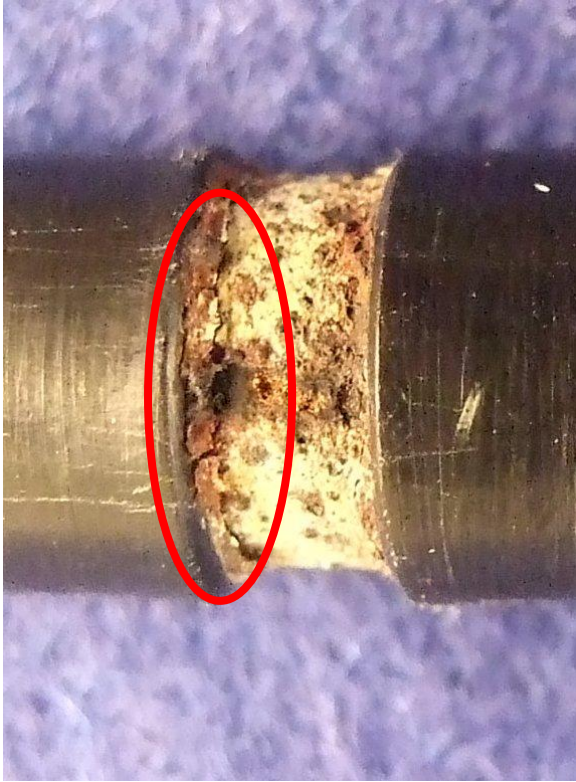
Figure 16. Cracks in the scale, in the area of severe corrosion.
