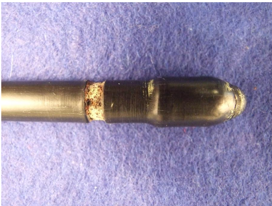
Figure 7. Test probe after exposure for 60 \text{ A/m}^2 AC and cp from a zinc anode.
