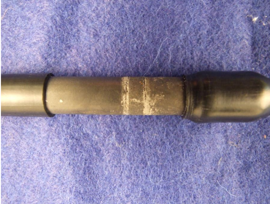
Figure 8. Test probe after removal of corrosion products.
