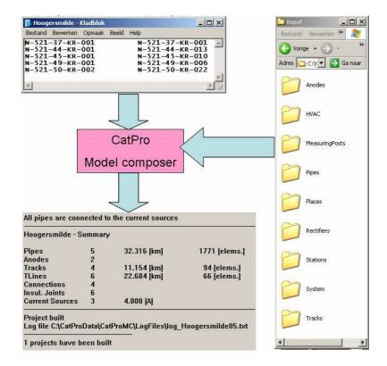
The section is 32 km in length and has two ground beds. One is near the rectifier and one in a remote area. The remote ground bed is used to model current from/to third party pipelines that are connected and to simulate 'current' defects. One can also see that the HVAC and DC traction geo-information is inserted in the model and that de MC has made 4 connections between pipelines and added 6 isolation joint.
