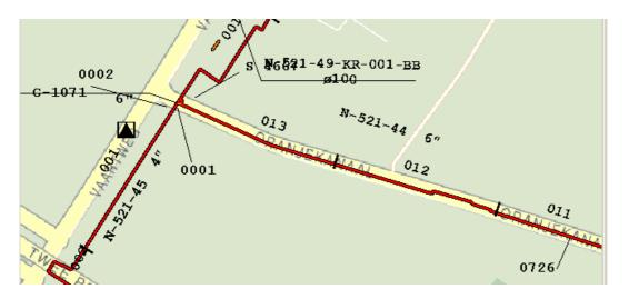
Example 2. Test post N-521-50-E0111 = Stand-by Test post N-521-50-E0072 = DC-interference (- - - = railway) and easy accessibly Test post N-521-50-E0071 = Stand-by annually, but measured in the 3 and 6 year program.
