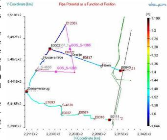
In this phase one can decide that the present chosen configuration is incorrect and needs to be changed. If the potential criterion is reached the conclusion is that the CP-system should be capable to apply sufficient CP to the pipeline. In this case the conclusion is "no problem".
