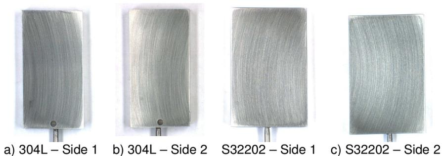
Figure 8: Pictures of surfaces after 1 month immersion test in 1 000 ppm chloride ion solution at pH 4.5 and 25°C
