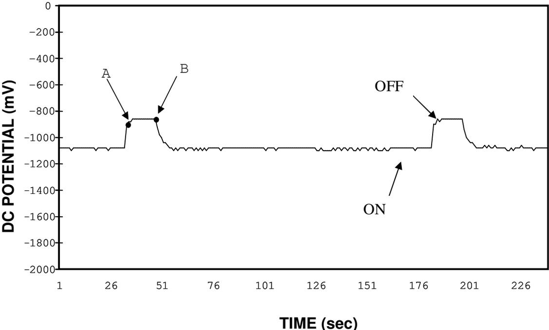
**Figure 1. On/off pipe-to-soil potential waveform—No capacitive ac-mitigation devices are connected - Test post KG 47.3 km,  $U_{ac}=13,8V$ .**
