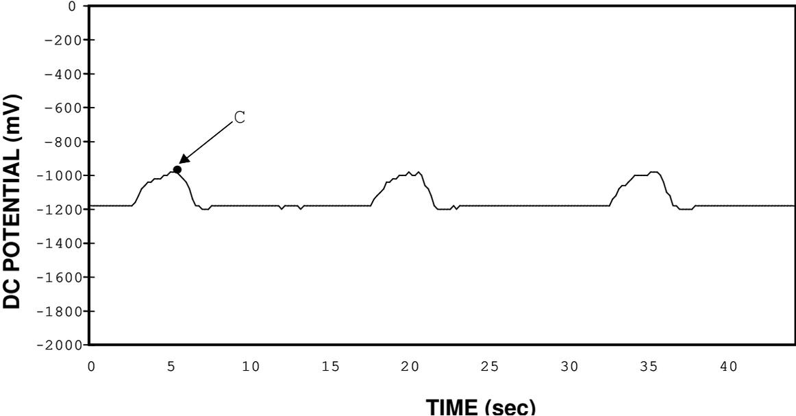
**Figure 2. On/off pipe-to-soil potential waveform—Capacitive ac-mitigation devices are connected -Test post KG 47.3 km,  $U_{ac}=1V$**
