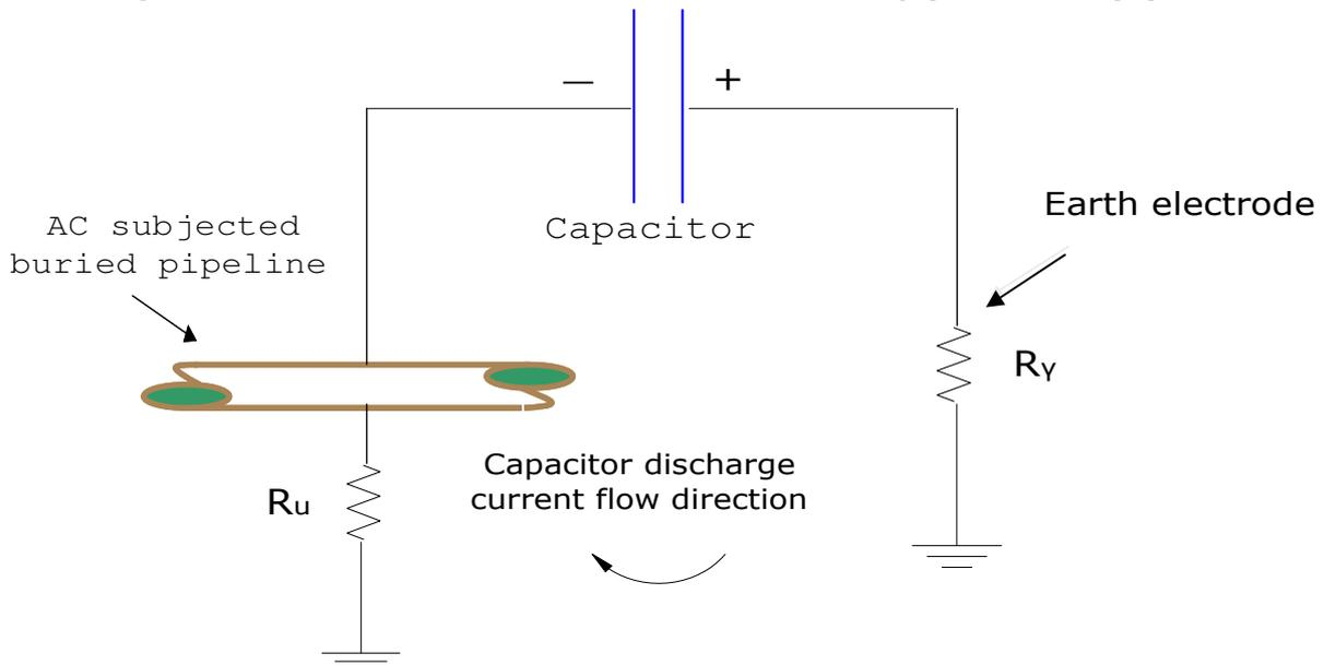
**Figure 4. Schematic of a cathodically protected pipeline connected to ground via a capacitor**
