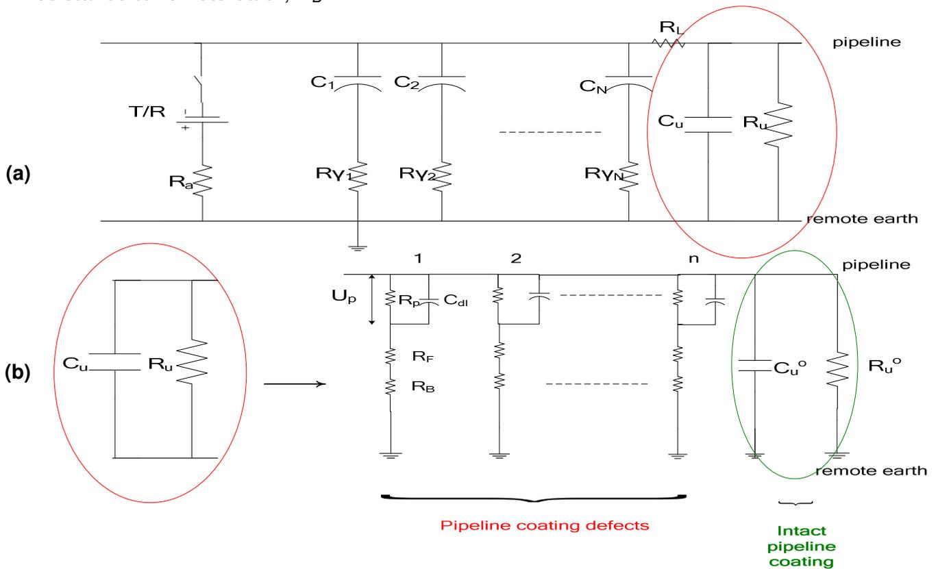
(a) circuit illustrating  $N$  ac-mitigation devices of capacitance value  $C_i$  each with earth electrode resistance  $R_{Y_i}$ , whereas  $C_u$ ,  $R_L$  and  $R_u$  illustrate the equivalent circuit of the pipeline itself. (b) circuit representing the buried pipeline based on coating defects with population number  $n$
