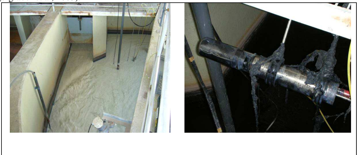
Figure 1: Measuring point gritchamber (left) and in-situ UV-Spectrometer (right)
