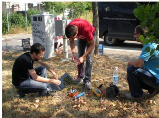
Tests have been performed using a Thinker and Razor datalog, a Volt meter, a dummy load to simulate AC interference and then comparing the readings with the Hyperdrone readings
