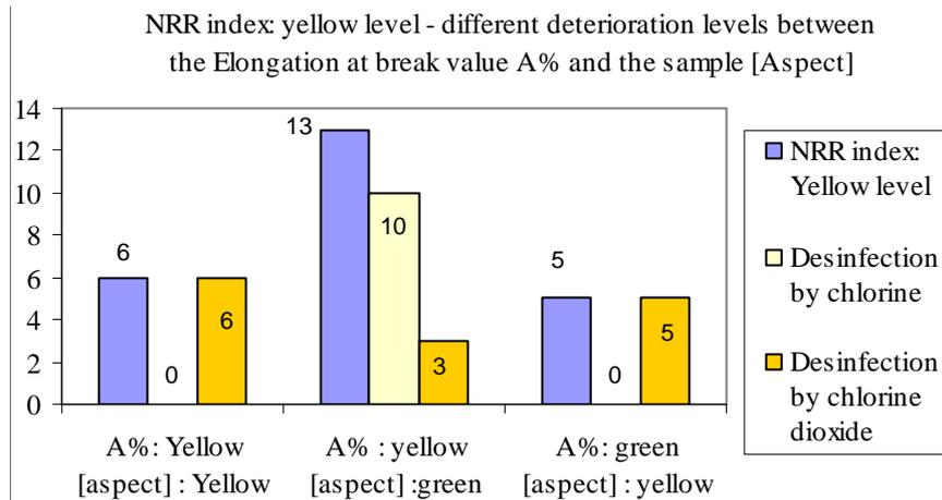
**Figure 12. NRR results – Yellow Level / Moderate degradation : repartition according to the disinfectant process and distinction between [aspect] and A%**
