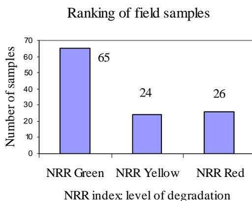
**Figure 7. Screening according to the NRR index obtained by the Nol Ring test**
