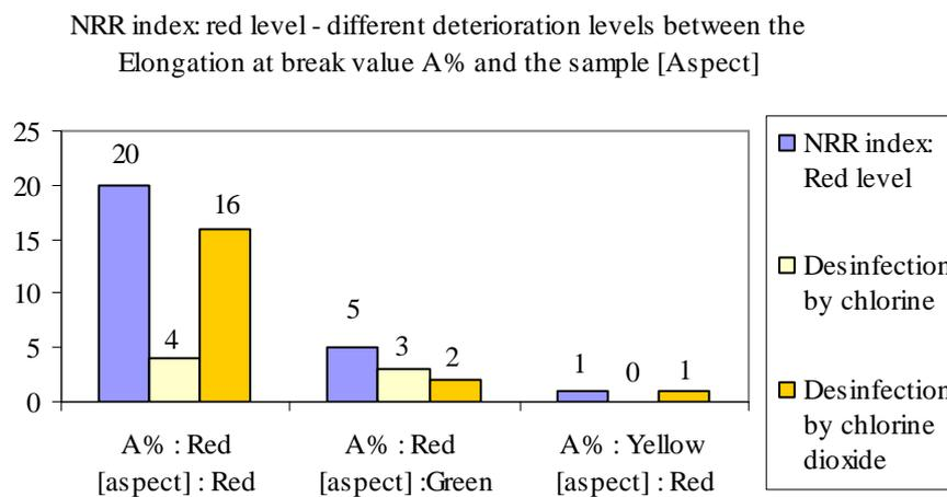
**Figure 13. NRR results – Red Level / High degradation : repartition according to the disinfectant process and distinction between [aspect] and A%**
