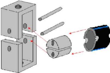
**Figure 2: Nol ring test fixtures**
