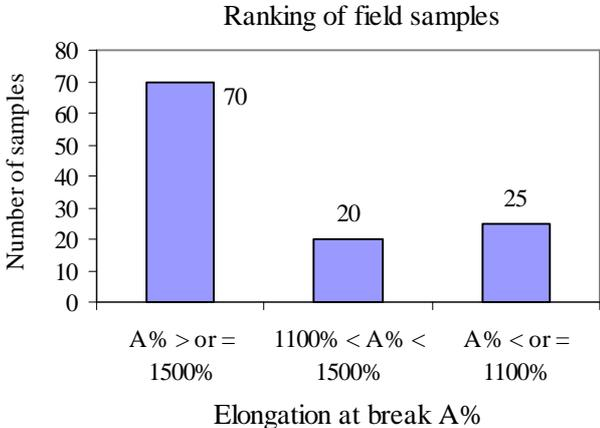
**Figure 7. Screening according to the Elongation at break value obtained by the Nol Ring test**
