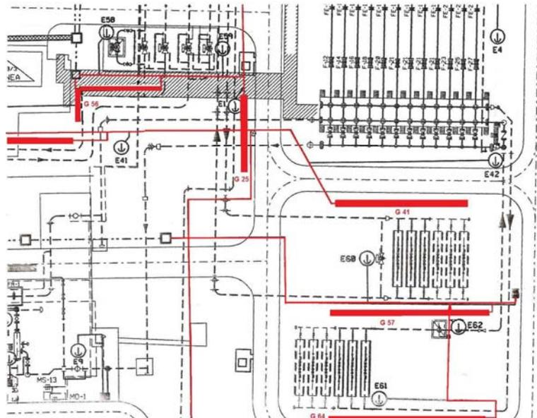
G = Groundbed, NM = Negative measuring cable, NP = Negative Power cable , E = Permanent Reference Electrode
