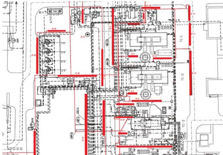
G = Groundbed, NM = Negative measuring cable, NP = Negative Power cable , E = Permanent Reference Electrode
