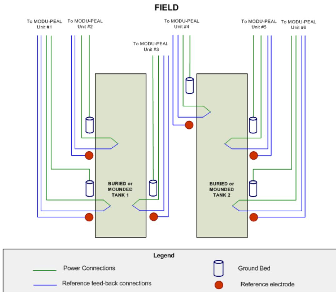
**Figure 1 – MODU-PEAL schematic connections to the field and to the wireless remote control system**
