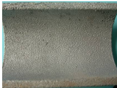
e) Galvanized steel coupons
