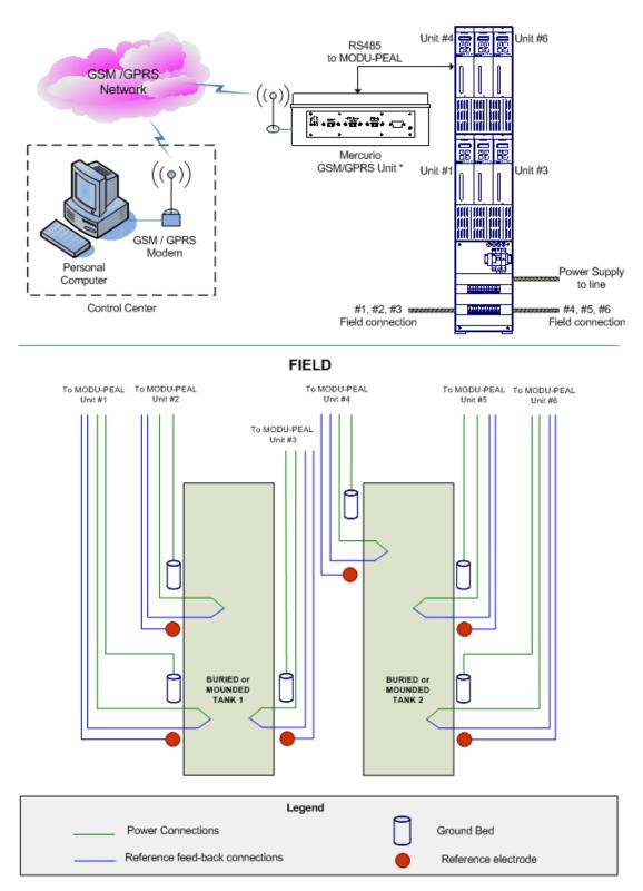
Figure 1 – MODU-PEAL schematic connections to the field and to the wireless remote control system
