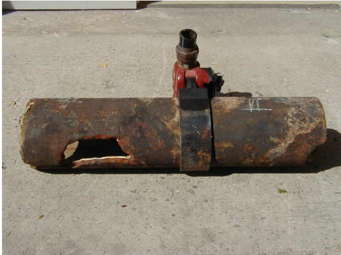
Figure 4: Corrosion damage of an old cast iron pipe
