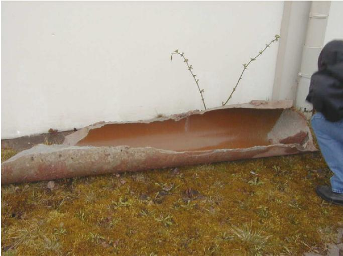
Figure 6: Corrosion damages of a cement asbestos pipe
