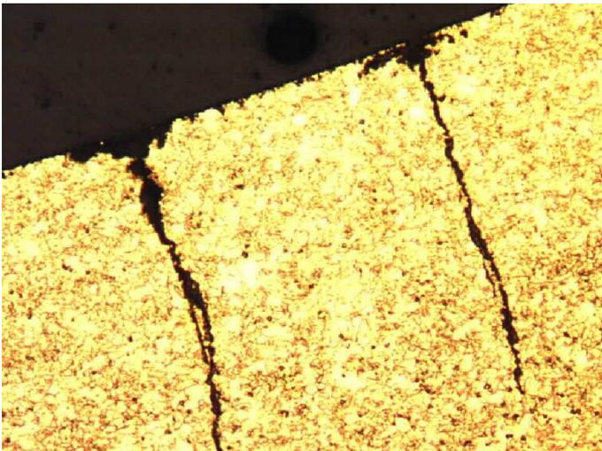
Figure 7: Stress corrosion cracking
