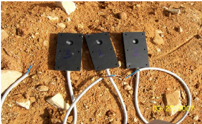
Three new a.c. Corrosion Coupons
