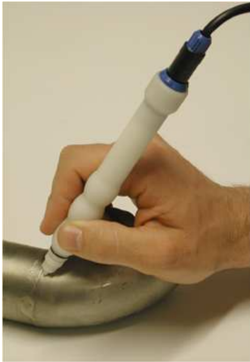
Fig. 1: Electrochemical measurement with the ec-pen on a stainless steel tube.
