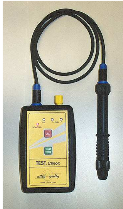
Fig. 2: Handheld instrument for quality control on stainless steels.
