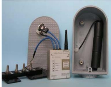
The CPW Unit is a very low power consumption equipment: three 1.5V alkaline size “D” batteries assure three years of operation with a daily GSM connection.
