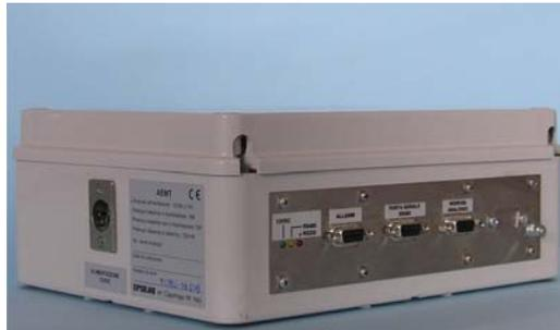
This equipment is designed to allow the remote control of one or more cathodic protection power supplies. In addition to this feature the unit can acquire voltage and current measures.
