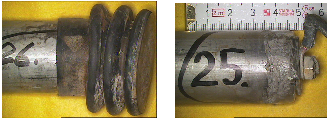
Figure 2. Test pipe of steel grade ASTM S32304/EN 1.4362 with intentional crevice under rubber sleeve. Left photo: before removal of the sleeve. Right photo: after removal – deep crevice corrosion attack (max. 1,3 mm) under sleeve.
