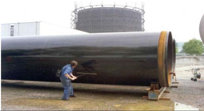
Figure 4: Holiday Testing with 25 KV (coating thickness 2,5mm)
