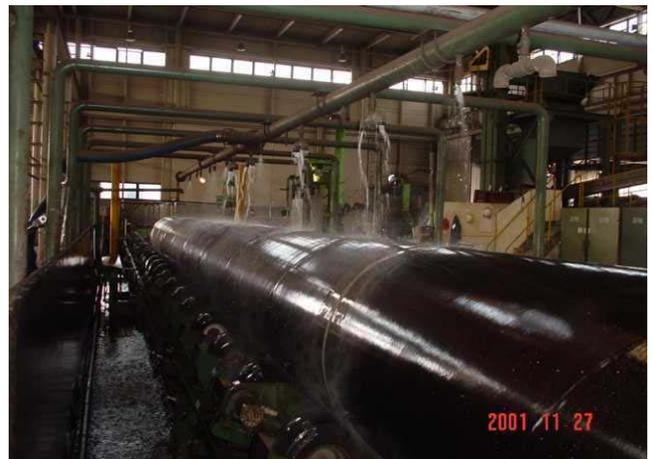
Figure 10: Online Coated Pipe - Cooling procedure at DYSP, Korea; PROTEGOL® 32-10
